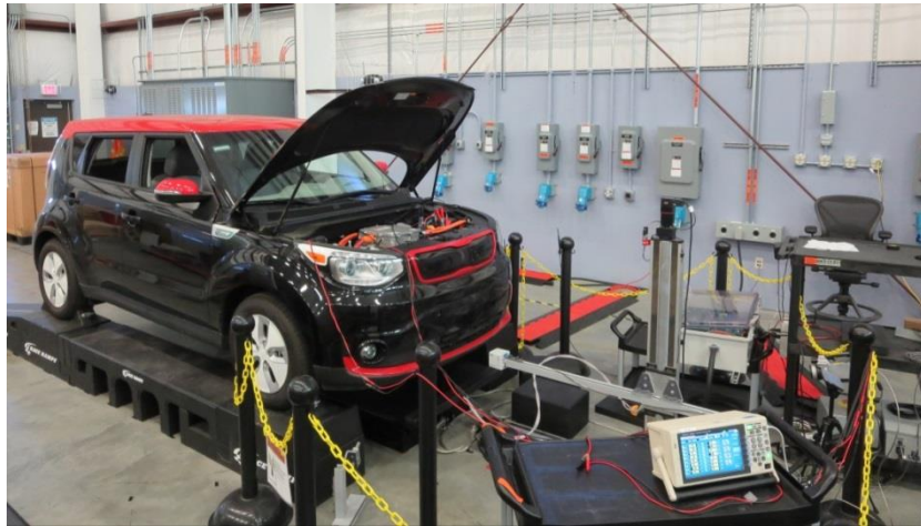
Figure 2. Hyundai / Mojo Mobility WPT system on Kia Soul EV during testing at INL's EVI lab
